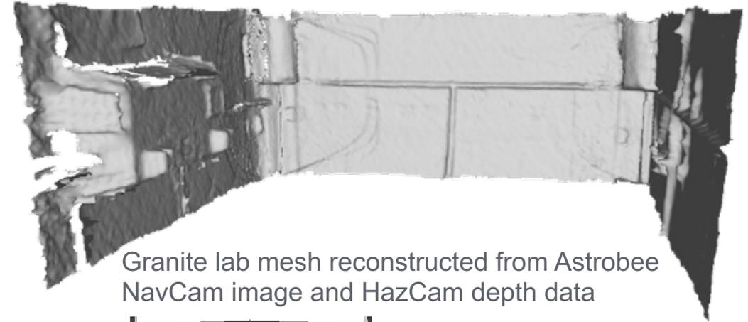
Granite lab mesh reconstructed from Astrobee NavCam image and HazCam depth data
