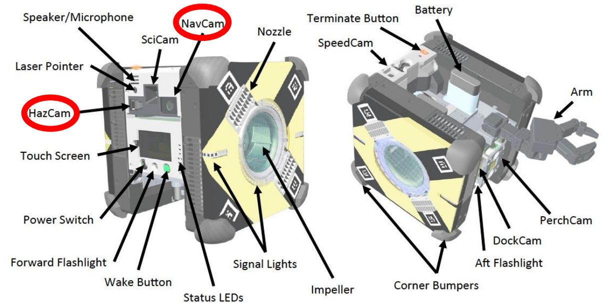
Astrobees are equipped with many sensors such as the HazCam and NavCam.
